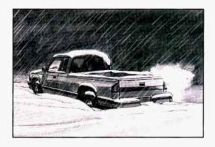
Run your engine only as long as you must. This saves fuel. When you run the engine, make it go a little faster than just idle. That is, push the accelerator slightly. This uses less fuel for the heat that you get and it keeps the battery charged. You will need a well-charged battery to restart the vehicle, and possibly for signaling later on with your headlamps. Let the heater run for awhile.
